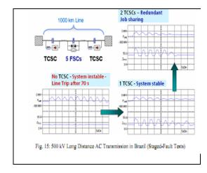
The recordings from on-site tests show that the interconnection would become unstable without the damping function of TCSC. If only one TCSC is in operation, the interconnection becomes stable, with both
